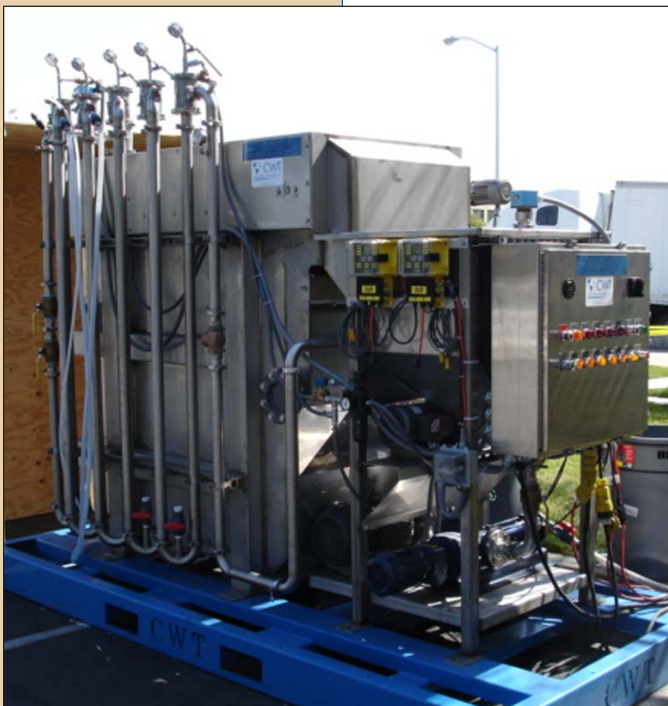
Figure 1 – Gem DAF Unit – Modular, compact and high efficiency
